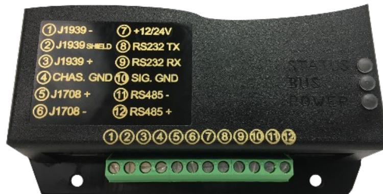
Figure 1: Procon<sub>TB</sub> Connector Pinout
